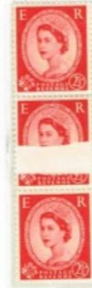
Web of paper has been thinned before printing, resulting in missing print on thin area of paper.
